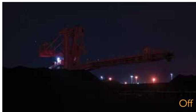
Improving energy efficiencies: Port Waratah installs LED lighting and smart ability to reduce lighting at night on major coal loading machinery when not required.
